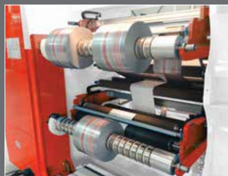
0-GRAVITY CONTACT ROLLERS TO IMPROVE THE PRESSURE ADJUSTMENT
